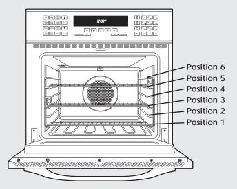
All ovens have six rack positions. Position 6 is the farthest from the oven bottom. Position 1 is the closest to the oven bottom. The racks can be easily removed and arranged at various levels. For best results with conventional baking, do not use more than one rack at a time. It is also recommended, when using two racks, to bake with the racks in positions 2 and 4 or positions 3 and 5.
